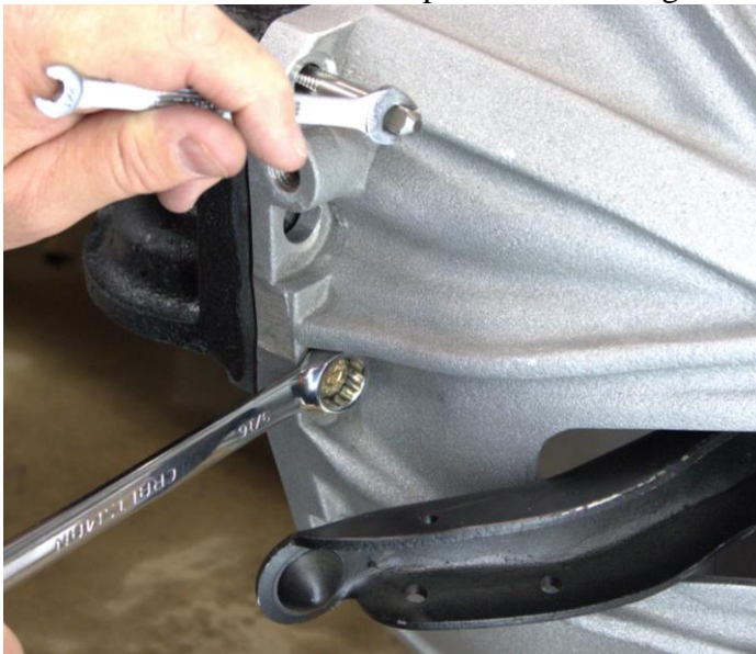
Removal of bolts and thread tap usage shown.
