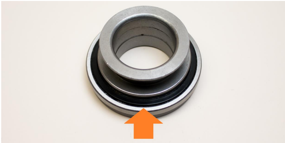
Seal Shown on the back side of the bearing, indicating constant-contact style bearing.
