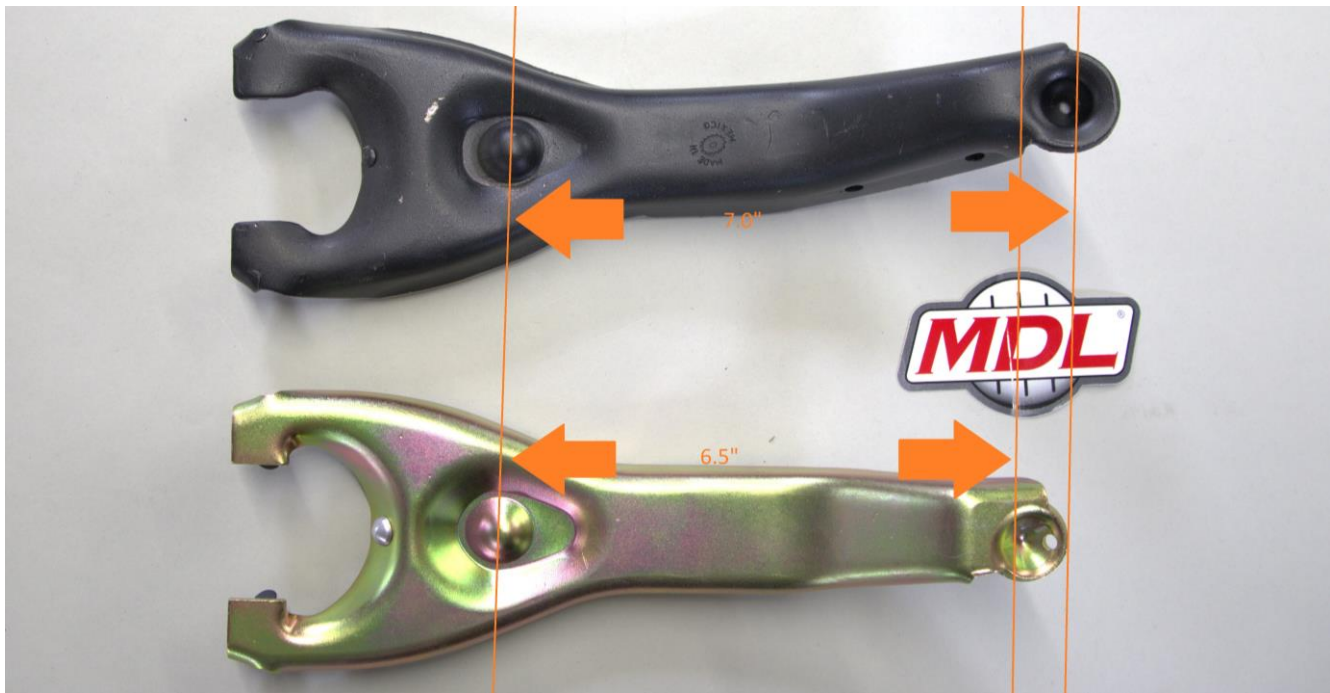
Center of fulcrum to center of dimple. Long and short dimple forks shown with dimensions.
